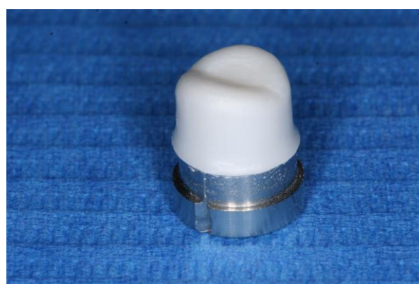
Figure 2. Zirconia coping cemented with a pressure of 20 N with the cement excess removed.
